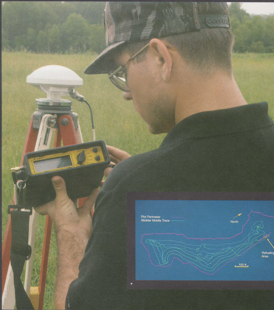
Agricultural engineers are using the U.S. satellite global positioning system to track the performance of forest machines. A researcher is shown testing a GPS receiver. The inset image shows the path of a skidder during herbicide spraying.
