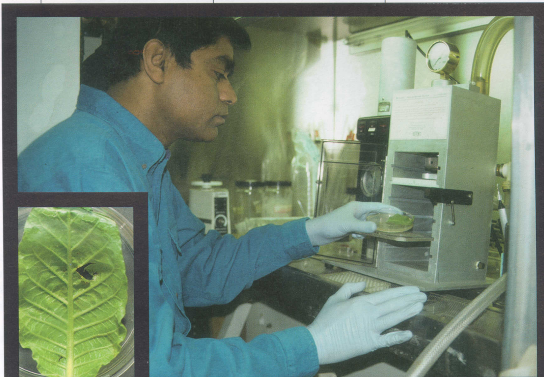
Molecular biologists are using a gene gun to blast foreign DNA into plant tissue, a procedure that allows them to perform genetic engineering studies not possible with traditional techniques. A tobacco leaf (Inset) is shown after it was bombarded by the device.
