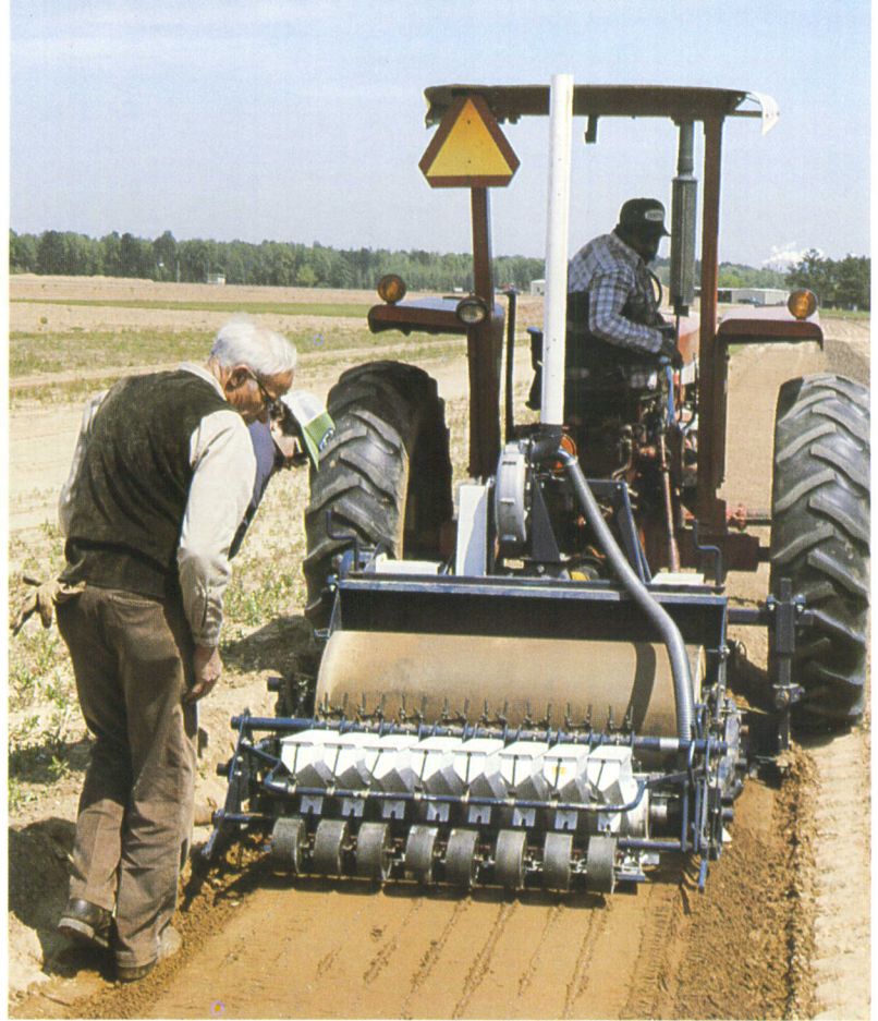
Use of a precision sower was found to increase seed efficiency by reducing the cull percentage.
