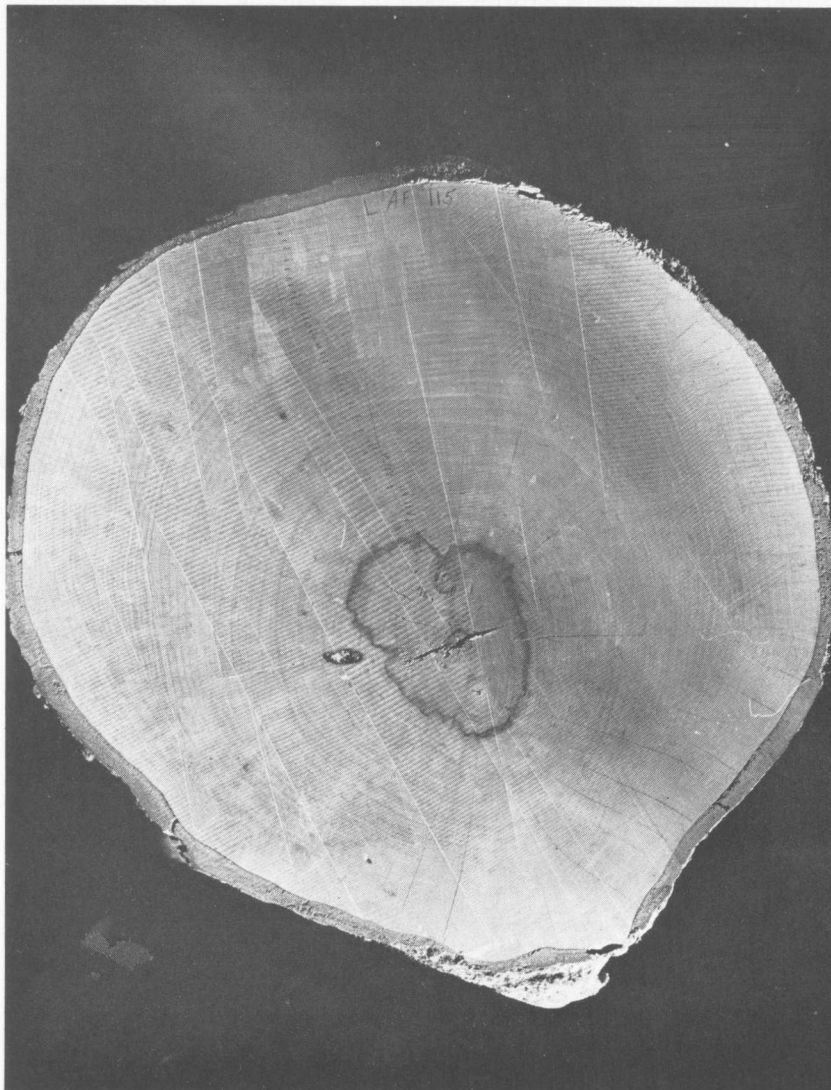
Figure 3. Transverse section of sweetgum that exhibited 6.2% discoloration. This small, central-column type discoloration is typical of stains initiated at limb stubs.
