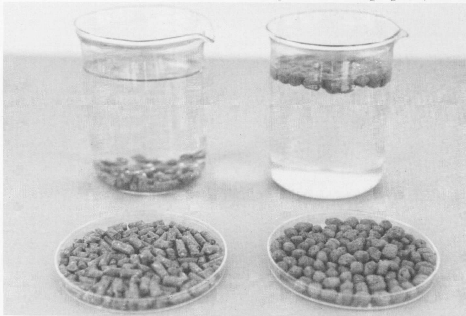
Extruded (floating) catfish diets (right) are made by cooking, expanding, and drying the ingredient mixture which requires more energy than the compression process for making pelleted diets (left).
