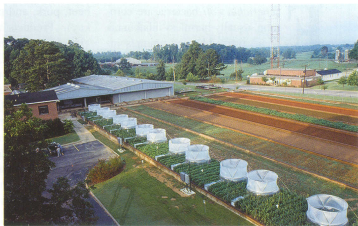
Open top chambers, used to generate large-scale CO 2 test atmospheres, during the first year of the sorghum and soybean study at the USDA-ARS National Soil Dynamics Laboratory. (Photo courtesy of Paul J. Hammock)
