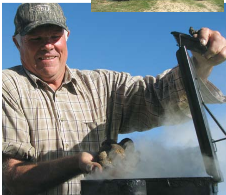
HORSE POWER —Renewable energy innovator Wayne Keith adds dry horse manure he found on the roadside in California's Death Valley National Park to the gasifier that fuels his Bio-Truck (inset).
