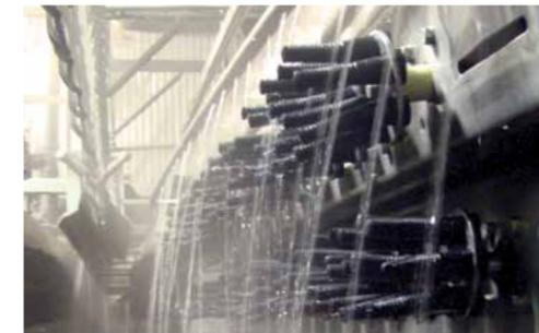
**FLOWING FREELY**—Water sprays from nozzles on a feather-picking machine at a poultry processing plant even though the processing line is idle. This plant has six pickers with a total of 252 nozzles. The Auburn water-use auditors concluded that leaving water running at the pickers unnecessarily wastes 18,182 gallons of water daily and 4.7 million gallons—and \$8,299—annually.
