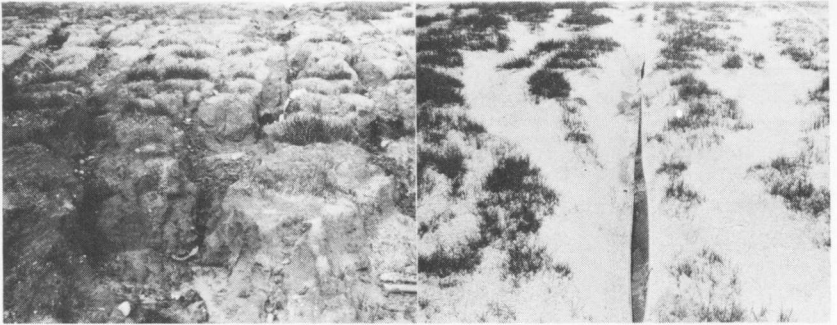
FIG. 5. Comparison of stands obtained on the Eufaula test site under no mulch (left) and Swift-Gro (right). Note that erosion occurred under the Swift-Gro netting.
