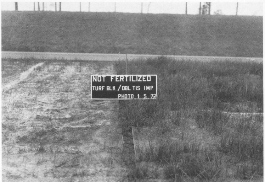
FIG. 3. Comparison of tall fescue seedling growth on plots mulched with Turf Blanket (left) and Swift-Gro containing plant nutrient adhesives (right) on a low fertility top soil in Baldwin County, Alabama.
