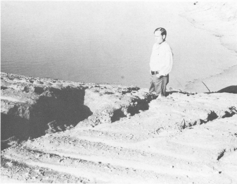
FIG. 4. Severe erosion which occurred on the Eufaula test site rendered most evaluations invalid.
