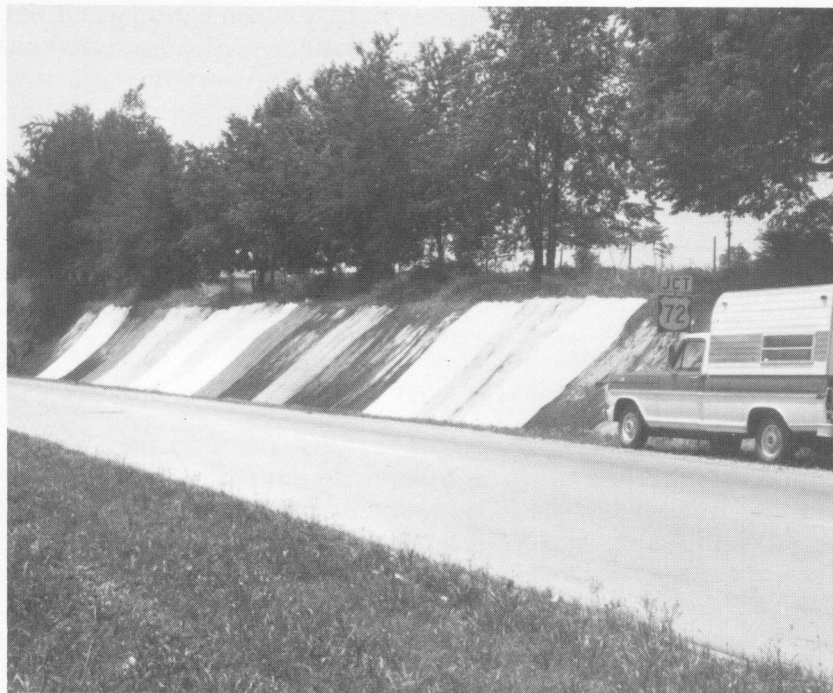
FIG. 1. General view of the west one half of the Athens test area immediately after application of mulches.
