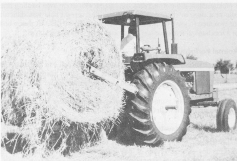
FIG. 2. (top) Two bales being transported with a tractor. NOTE: Front loaded bales should be transported close to the ground and at slow tractor speeds (see Highlights of Agricultural Research, Vol. 24, no. 2) (bottom) Round bale unrolling mechanism used in System 2.
