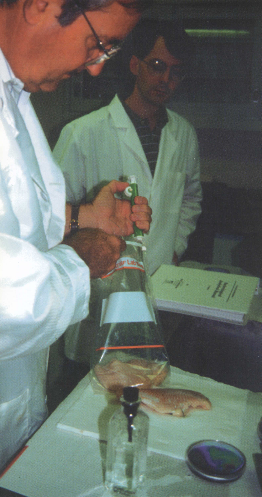
Catfish fillets are macerated in sterile phosphate buffered water prior to analysis for E. Coli.
