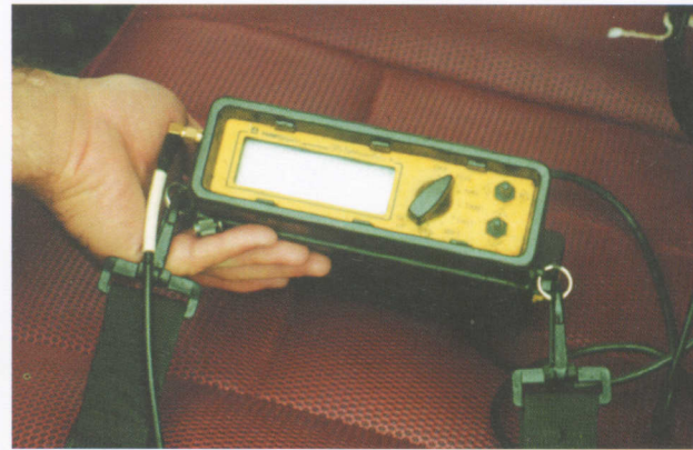
Figure 2. Hand held GPS receiver used to collect stationary and mobile GPS field data.
