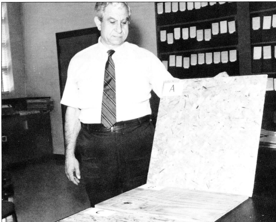
Test samples shown are (A) waferboard, (B) southern pine plywood, and (C) oriented strand board.
