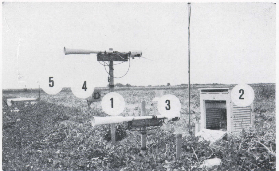
FIG. 2. Equipment used in monitoring environmental parameters at the Wiregrass Substation, Headland. Foreground: 1. air temperature sensors, 2. hydrothermograph in a ground-level weather shelter, 3. rain gauge; background: 4. volumetric spore trap, 5. anemometers.
