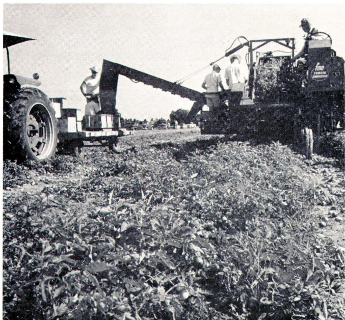
Close spacing of tomato plants proved necessary for highest yields when the crop was once-over harvested with this machine.
