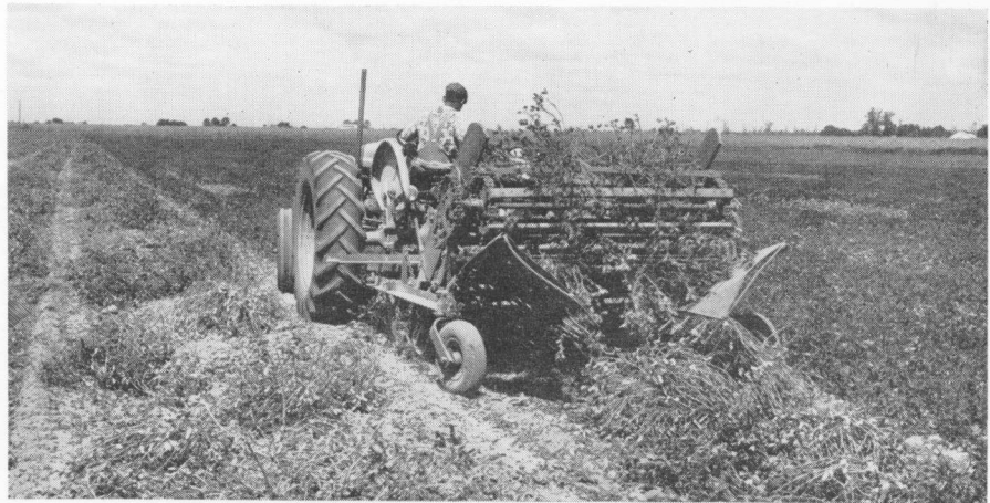
Mechanization of row crop production has been an important phase of research at the Wiregrass Substation. Peanuts have become the No. 1 money crop of the area as a result of efficient production. Digging and shaking by machinery in one operation, shown above, and combining have done much to bring about efficiency.
