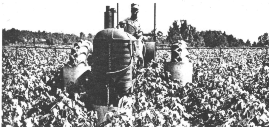
Tractor sprayer rig equipped with wheel shields to reduce injury to plants.
