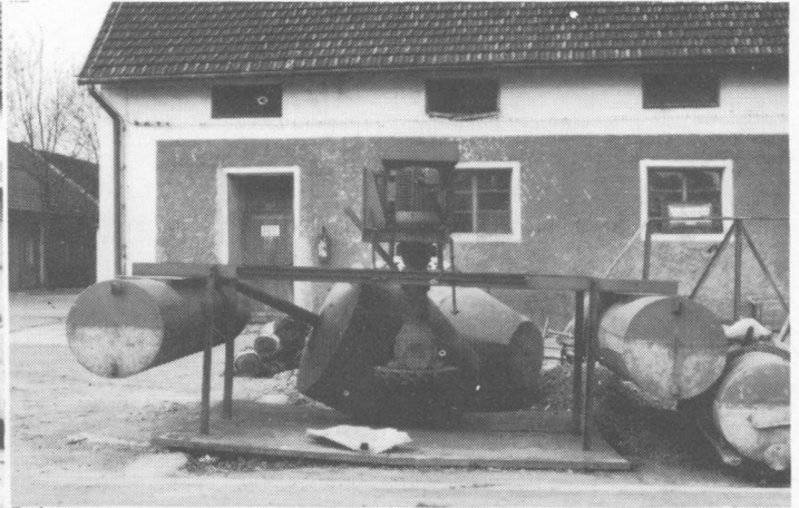
FIG. 3. Aerators, such as these which are electrically powered, are lately being used in carp culture ponds where more intensive culture is being practiced.
