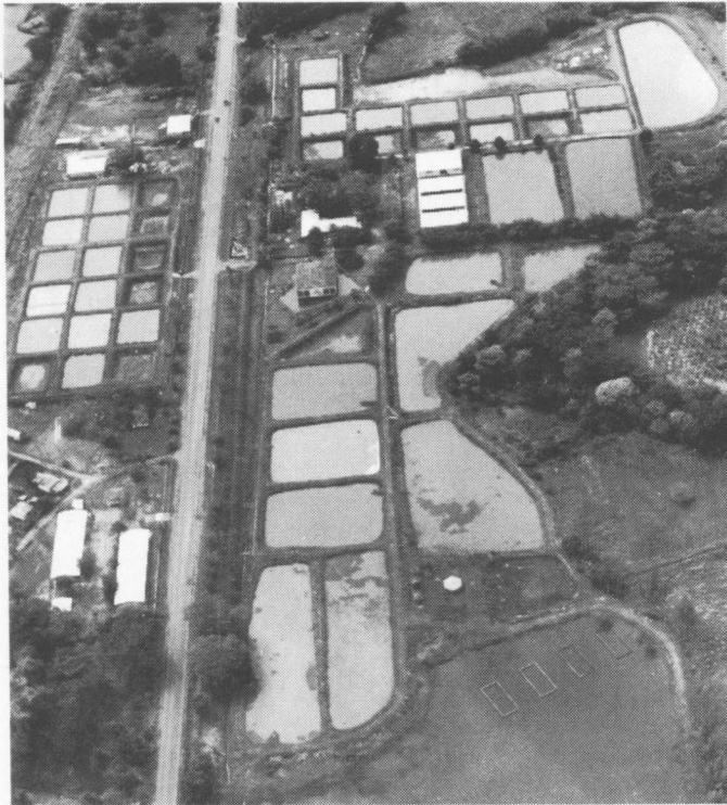
Aerial view of the National Fisheries Station, Santa Cruz Porrillo, after new construction was completed in early 1975. The station now has 30 concrete tanks and 32 earthen ponds for experimentation plus 15 earthen ponds for fingerling production. Total water area is 6.1 hectares.
