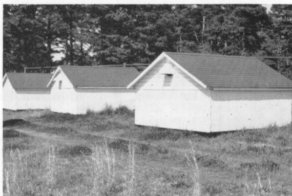
Shown here are three of the battery of various attic types under test at Auburn to determine best system for lowering house temperatures.
