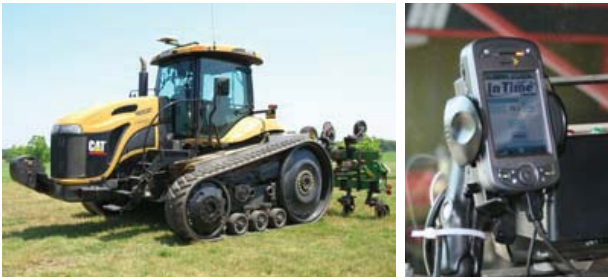
Figure 1. Tractor equipped with RTK GPS receiver and Internet accessible cellular phone, which receives real-time GPS correction signal from a CORS site in Lawrence County, Alabama.
