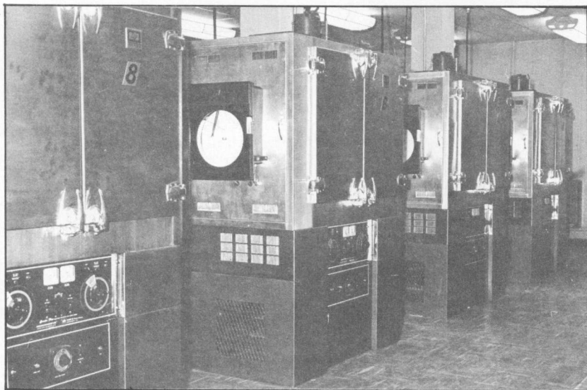
Fig. 1. Eight temperature/humidity cabinets were used to study the mold. Each cabinet had working dimensions of 37" wide by 19" deep x 25" high and was controlled by Duel Wet and Dry Bulb POWER-O-MATIC 60 Saturable Reactor Control Systems.
