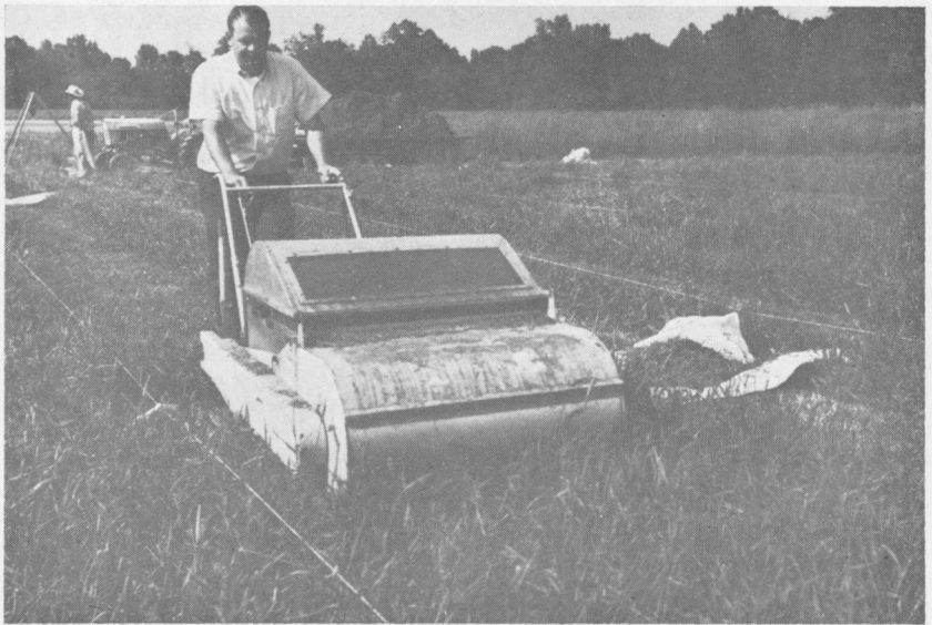
FIG. 1. Cool season perennial grass plots were harvested with this flail harvester, and forage from each plot was weighed for yield comparisons.
