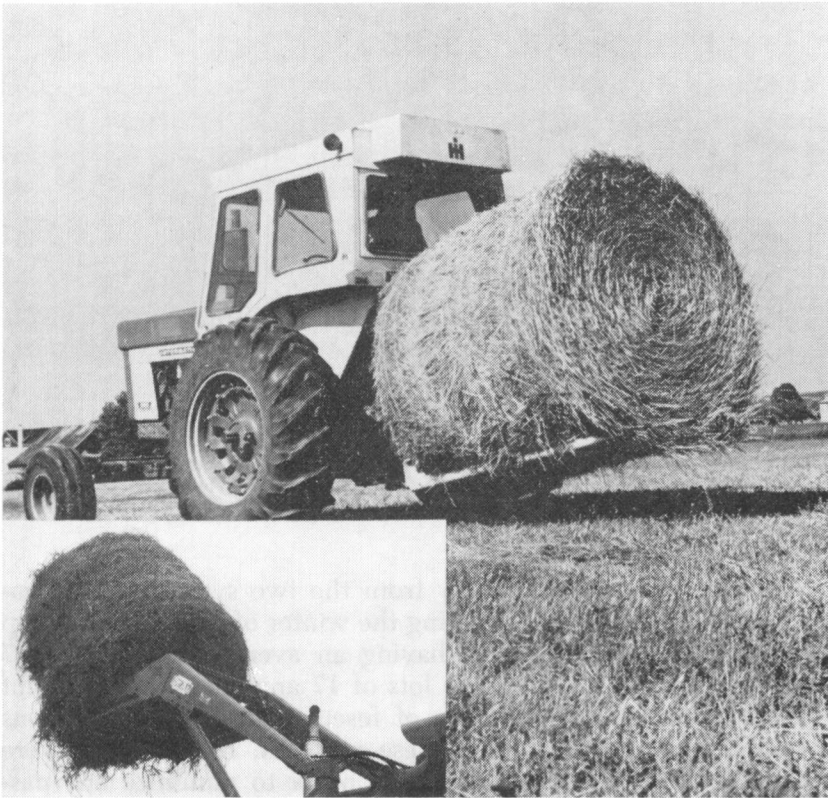
FIG. 2. Large round bales can be loaded on a truck or trailer for transport using a tractor equipped with a front-end loader or a rear-mounted loader. Capacity for the round baler system is greatly influenced by the bale transport system.
