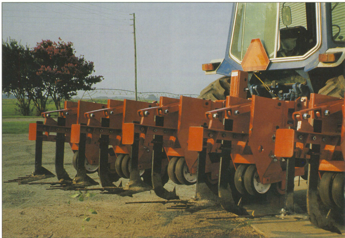
Brown-Harden Chiselvator showing sweeps with metal rods welded to trailing edges.
