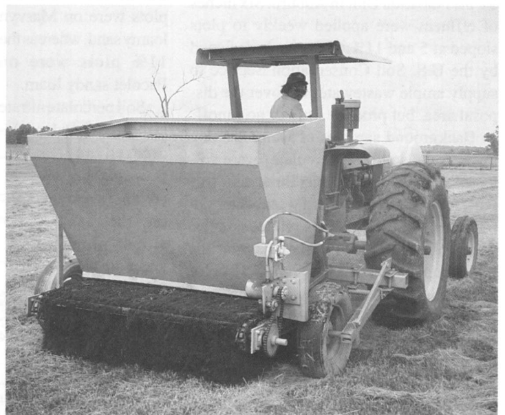
AAES drop applicator for spreading chicken litter and other organic solid wastes.
