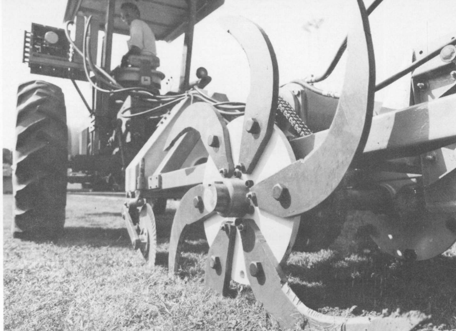
The field prototype of a powered rotary chisel in an early stage of its development (NTML Photo No. A10, 305a).
