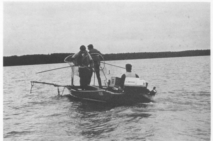
Fish populations in major reservoirs are sampled with the aid of electrical fish-collection equipment.
