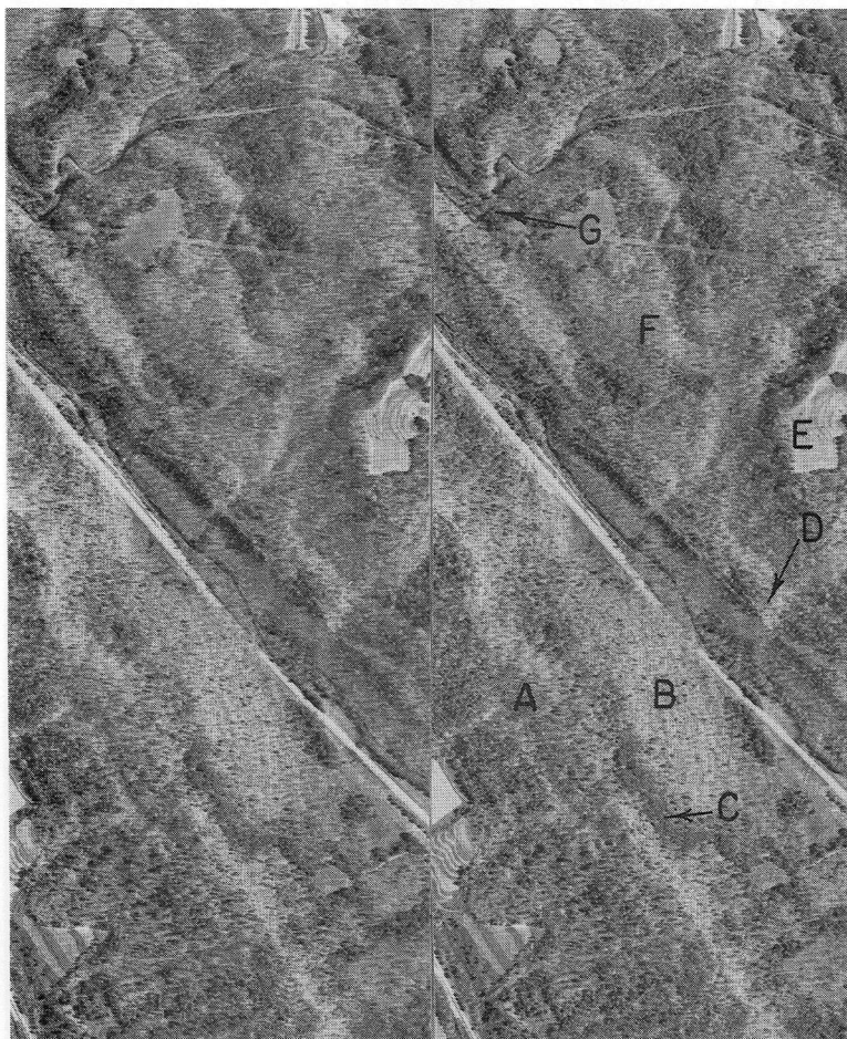
FIGURE 22. Stereogram of a portion of the Sequatchie (or Brown's) Valley showing the sequence of geologic strata. The western boundary ridge is Pottsville sandstone (A). The east facing slope of the ridge is Bangor limestone (B). Sandstone talus extends down-slope varying distances. (Pine occurs where sandstone talus is present as at (C)). The contour-line-like striations at B are good evidence for the presence of limestone, as is the absence of pines. The dark crowns on the limestone are eastern redcedars. The Hartselle sandstone can be seen as an almost vertical dike-like structure at D. It also forms the nearly horizontal field at E. The jumbled hills east of the Hartselle sandstone ridge are Tuscumbia limestone and Fort Payne chert (F). The stream at G is approximately 15 feet wide, the critical stream width in the Warrior Basin Forest Habitat Region. (Blount County, GP-4LL-4,5).
