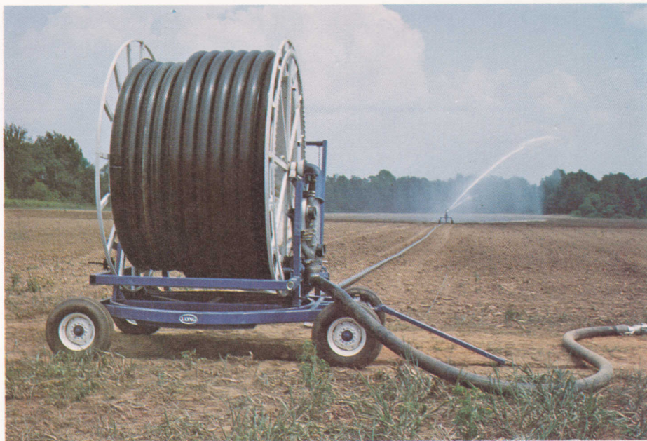
The problem of non-uniform watering by hose-towed irrigators, caused by speed variations as the hose is wrapped around the takeup drum, is getting attention in Auburn research.
