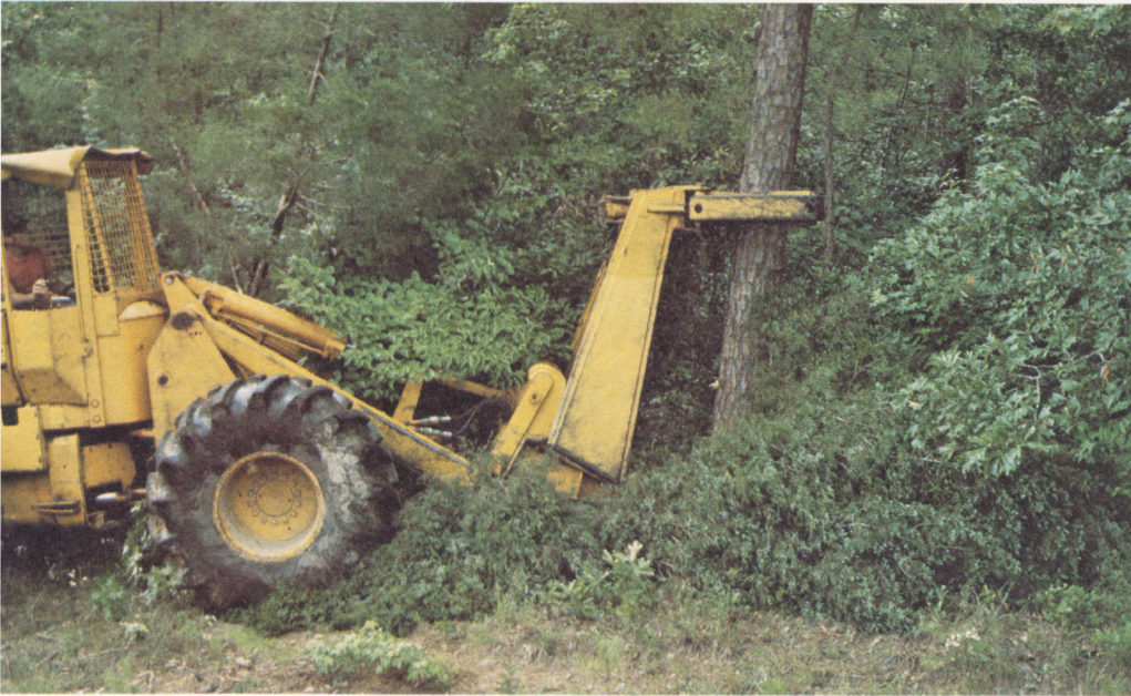
Six brands of feller-bunchers were evaluated on 10 logging operations during the year, with attention given to tree size, slope, and ground condition effects on performance.
