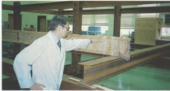
Development of I-beams, currently in demand from builders, provides more efficient use of Alabama's forest resources.
