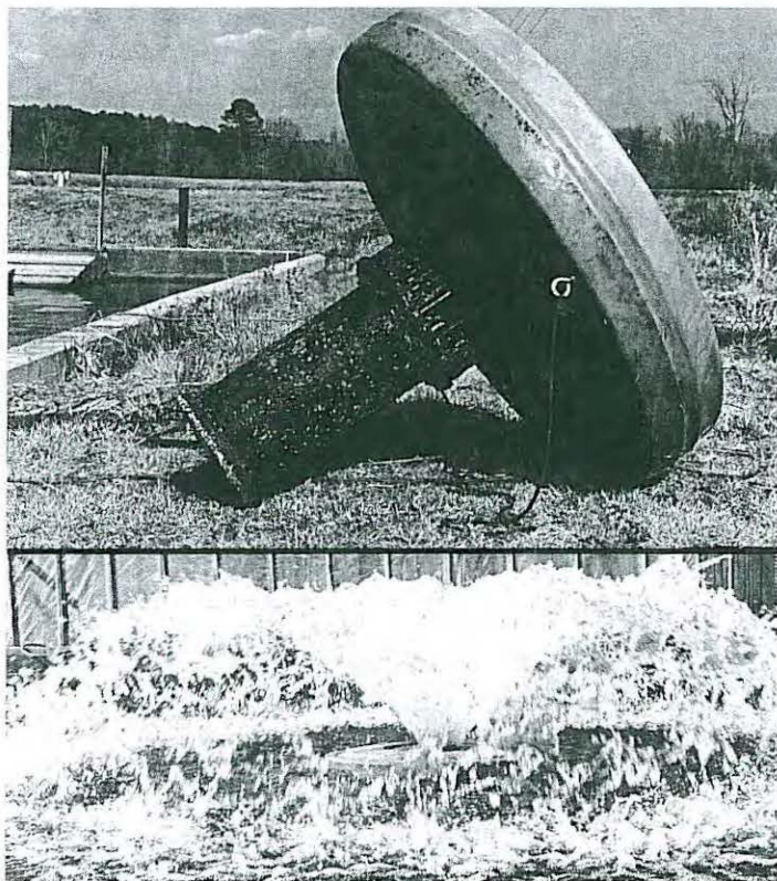
Figure 17. Vertical pump aerator.
