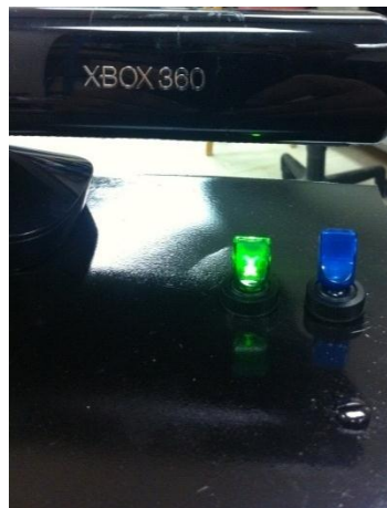
Figure 16. Shows both switches in the ON position for cart to begin commands.
