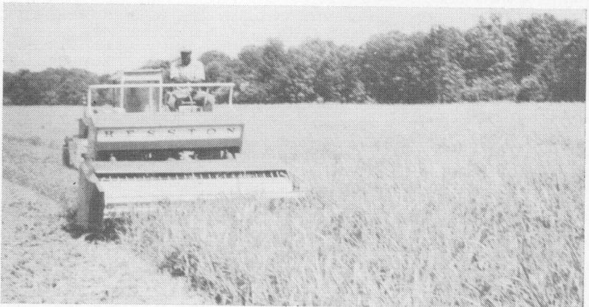
FIG. 1. Johnsongrass for the hay studies was cut and conditioned in one operation. Raking was a separate operation.
