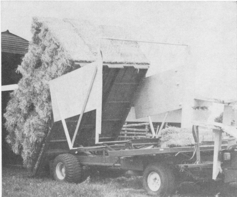
FIG. 5. Bales are stacked for storage by same machine used to load and transport them.
