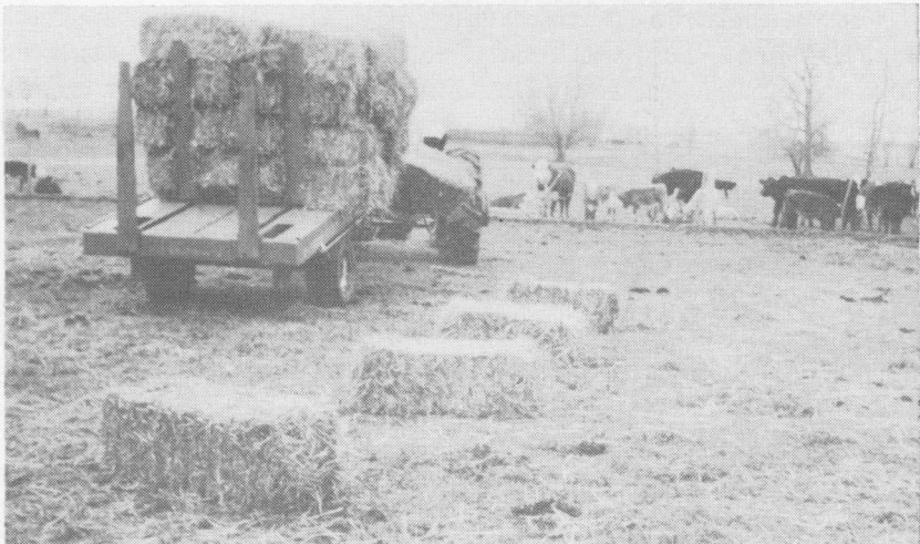
FIG. 10. Feeding bales with a bale wagon. Bales are discharged from the machine one at a time. Bale twine was not removed for feeding.
