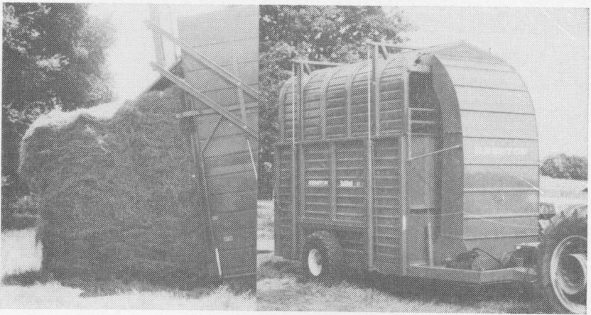
FIG. 3. On the right is a machine used to produce stacks of hay. Left shows stack being discharged from machine at the storage area.
