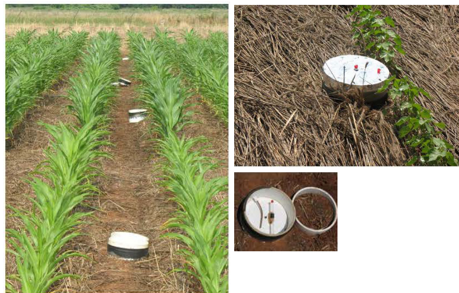
Figure 1 (left) Placement of static chambers used to collect ammonia volatilized in selected treatments; (top right) A heavy residue cover in 2008 may have enhanced ammonia volatilization losses from UAN solution sprayed on the top. Agrotain® did not seem to reduce losses under these conditions; (bottom right) Static chamber.
