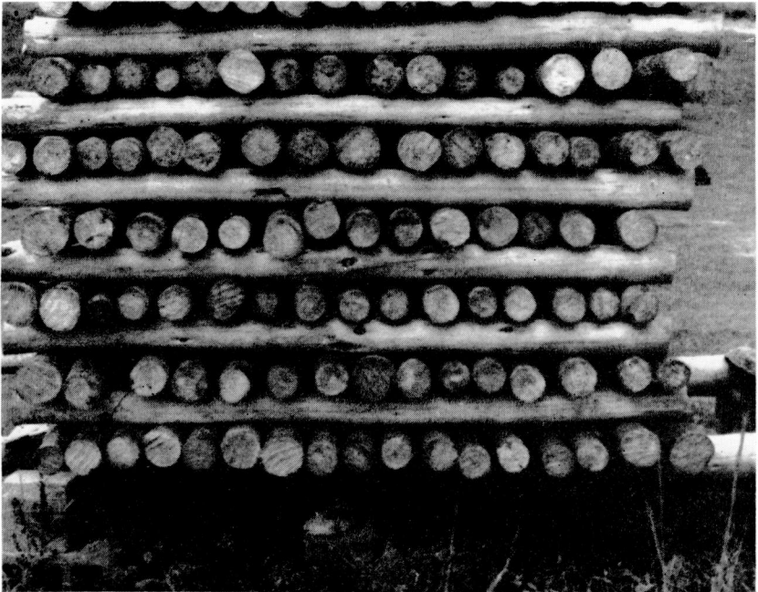
FIG. 8. These posts are stacked too close for proper seasoning.
