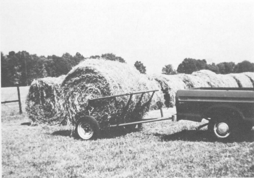
FIG. 2. Low-cost single-bale hauler. Trailer requires some hand labor for loading and can be pulled by a truck or tractor.
