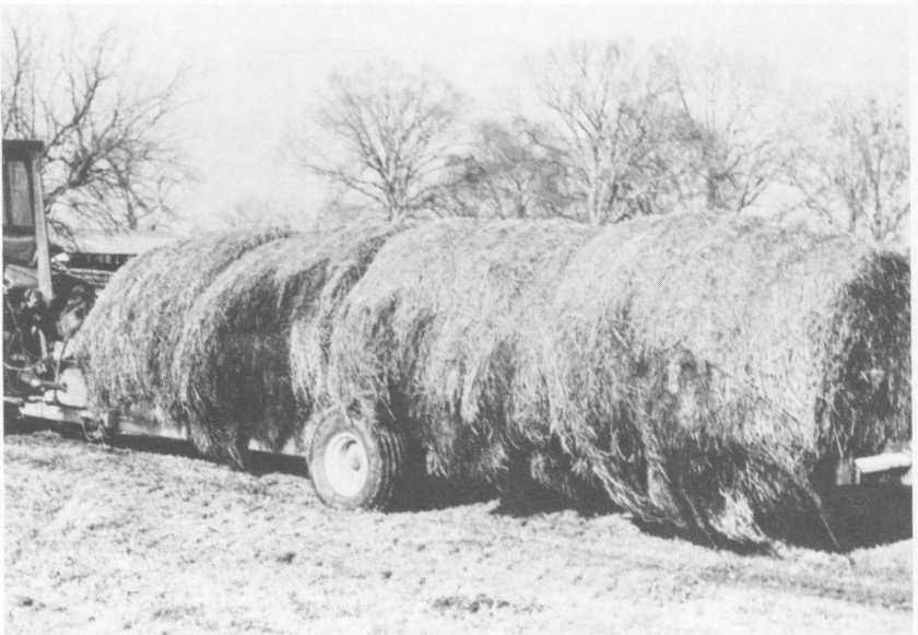
FIG. 4. Bale transporter hauling four bales. Machine loads and unloads bales one at a time.
