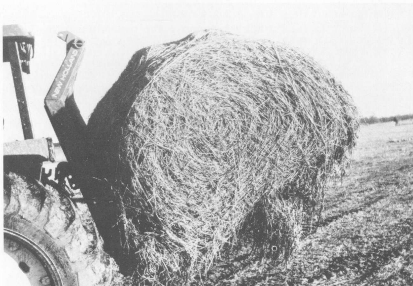
FIG. 1. Rear-mounted 1-bale hauler on a farm tractor. Additional front-end weight should be used to counterbalance the bale.
