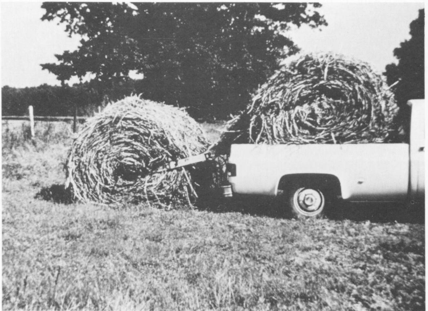
FIG. 3. Pickup truck equipped with mechanism to self load and unload round bales. Operator controls are located in the cab.
