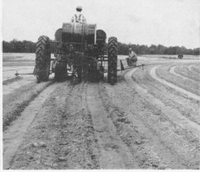
Cotton can be planted and pre-emergence weed control chemical applied in same operation with sprayer mounted as shown above. Note the well-prepared seedbed and use of row marker and wide press wheel.
