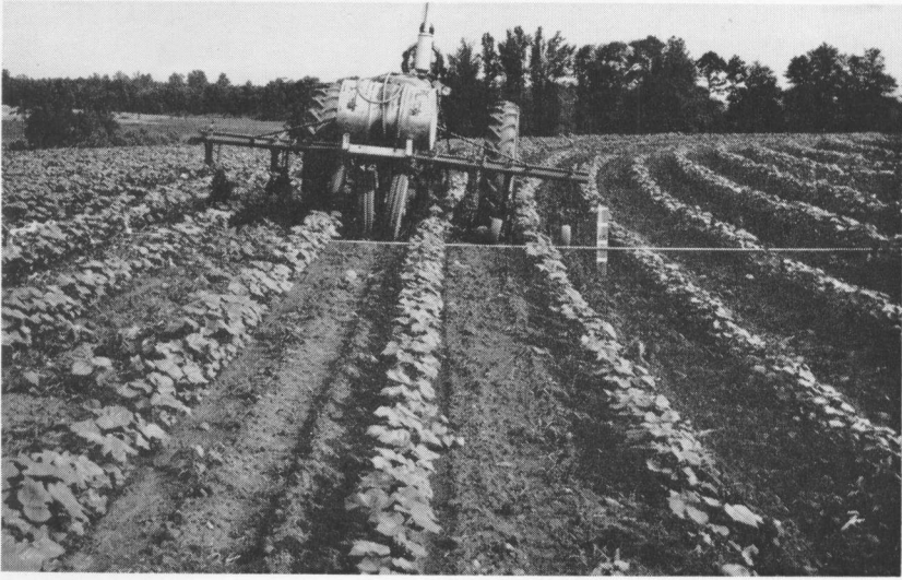
This four-row cultivator is being used on a broad terrace built for mechanization. Line in foreground shows cross section of broad terrace channel.
