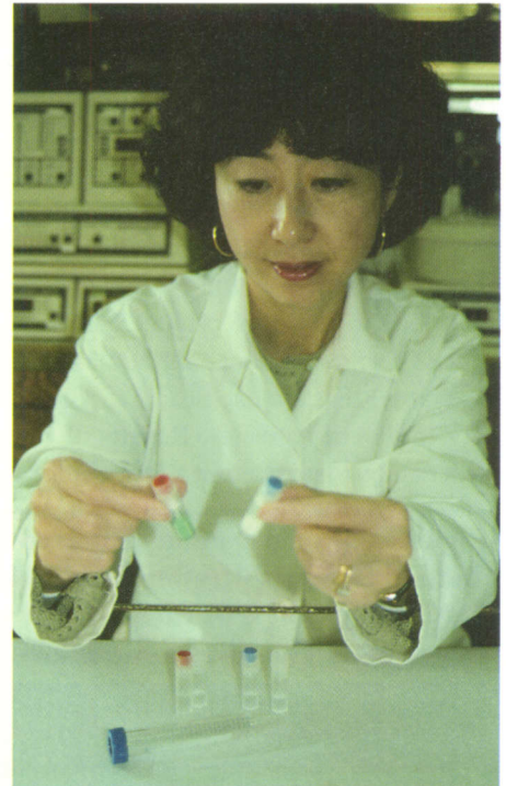
Hsieh displays AAES-developed test kit used to detect meat species in processed meat products.
