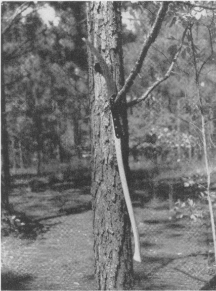
FIGURE 4. Shown here is the Maylan saw, which was especially designed to prune trees in forest stands. It is highly recommended for this purpose.
