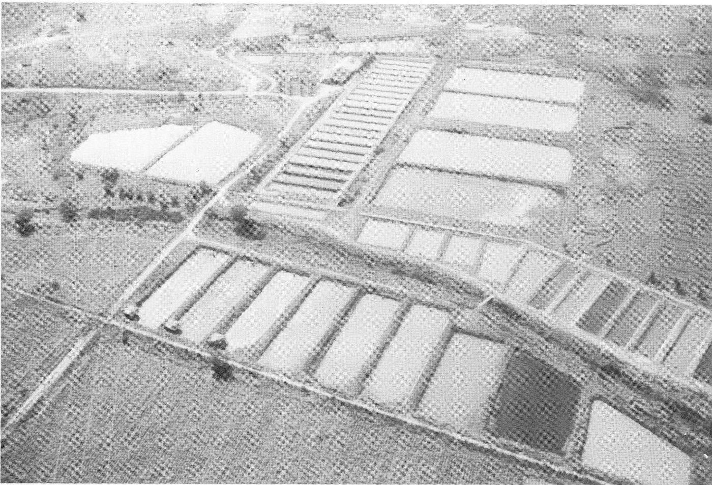
Phase I of Rodolpho von Ihering fish culture research center in Pentecoste, Brazil, provides pond facilities for fish culture training and research. Note pig sties constructed over the ponds in lower left corner of photograph.
